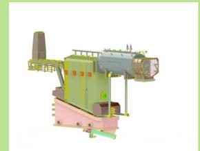
Today's environment requires a high degree of flexibility to choose the type of Biomass and other solid fuels. The GETABEC Dynamic Step Grate combustion technology combines flexibility with high efficiency. The GETABEC Dynamic Step Grate is designed with 4 combustion zones. Each zone is controlled independently to ensure the correct fuel / air ratio and the mechanical rotation of the fuel. This process will allow the highest possible efficiency of the combustion system.
